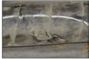
Hole in hose cover that exposes reinforcement
