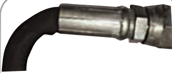
Hose bent too tight, damaged at end of coupling
