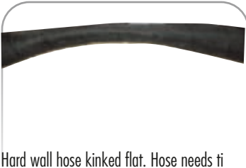
Hard wall hose kinked flat. Hose needs to be replaced.
