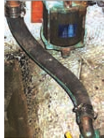
Clamps installed with screw tightening heads in line. It is recommended to offset as see below.
